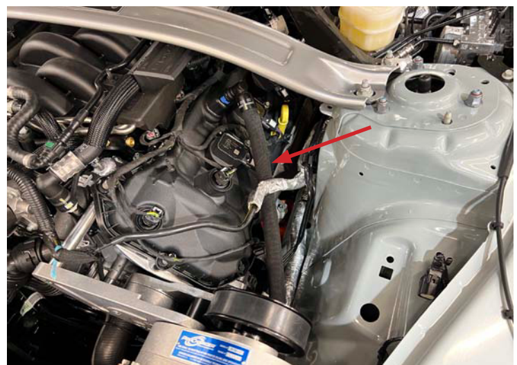
PCV Line Installed
