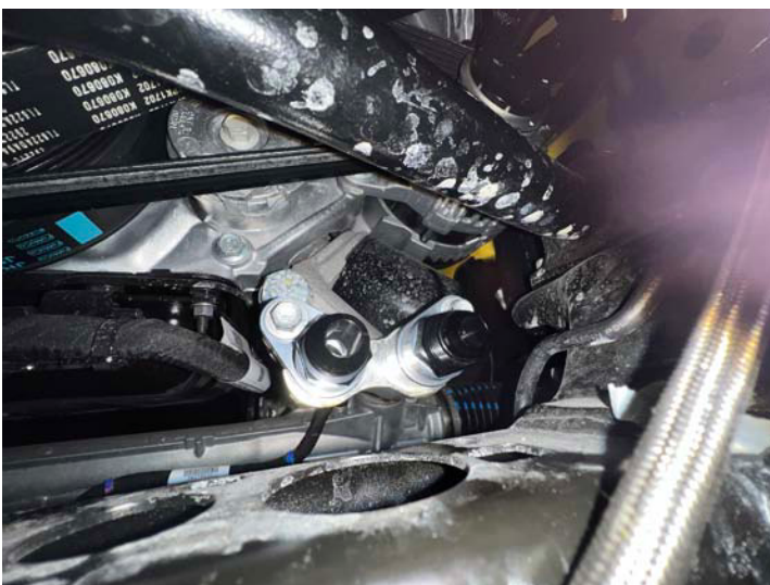
Oil Cooler Adapters Installed
