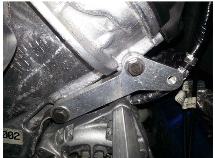
Sub Bracket Installed
