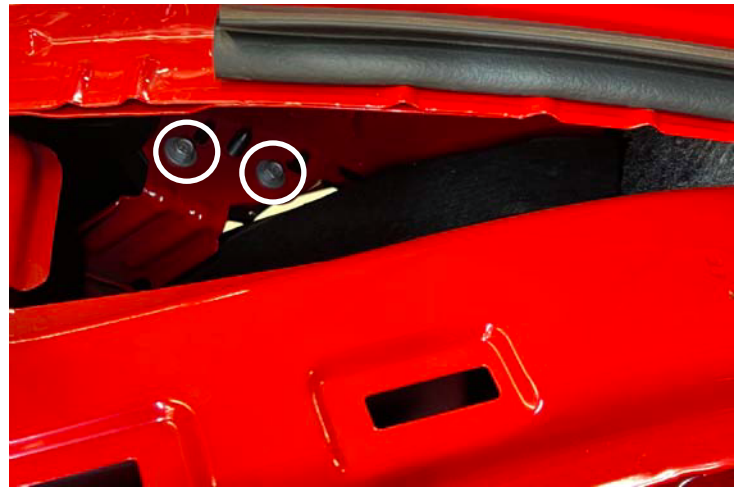
Fascia Corner Bolts
