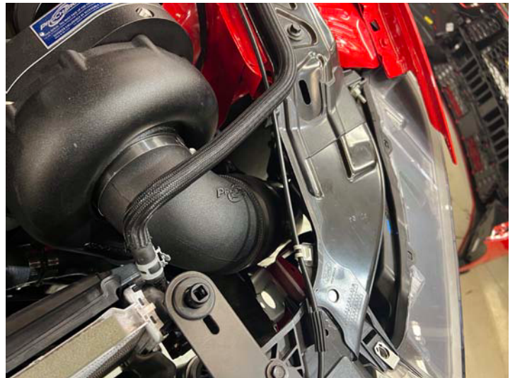
Rotomold Inlet Installed
