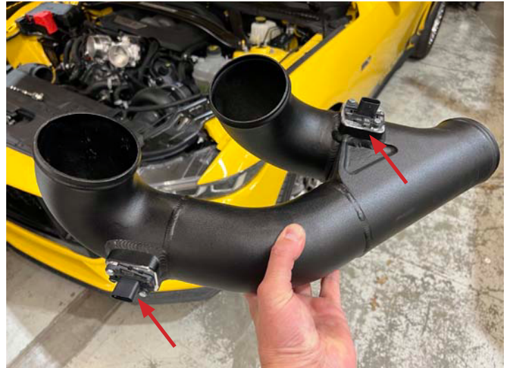
MAF Sensors Installed
