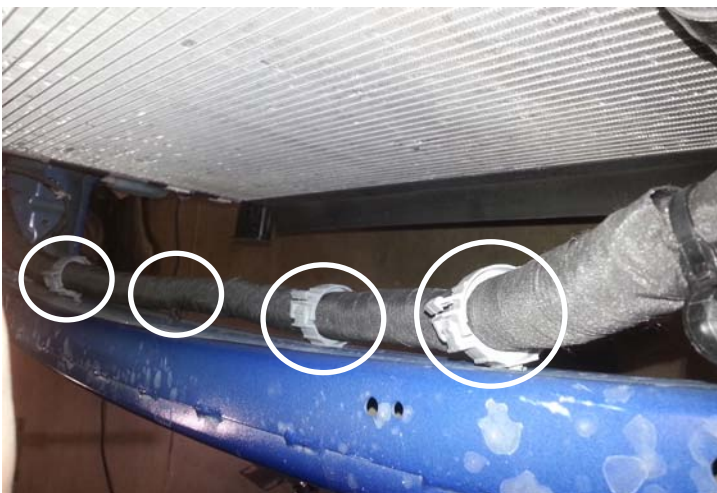
Wiring Harness Retainers
