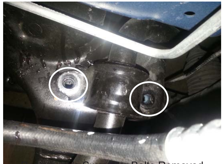
Passenger's Sway Bar Bolts Removed
