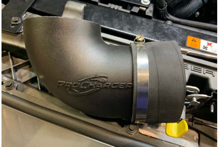
Plastic Inlet Installed
