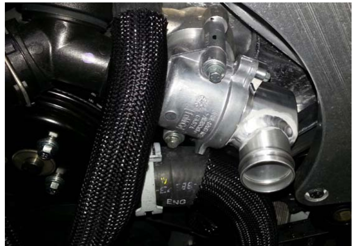
New Thermostat Housing Neck Installed
