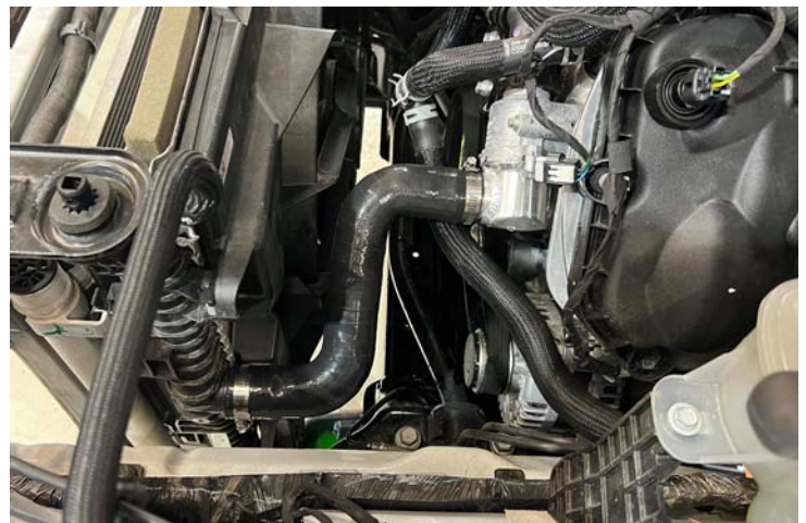
Lower Radiator Hose Installed
