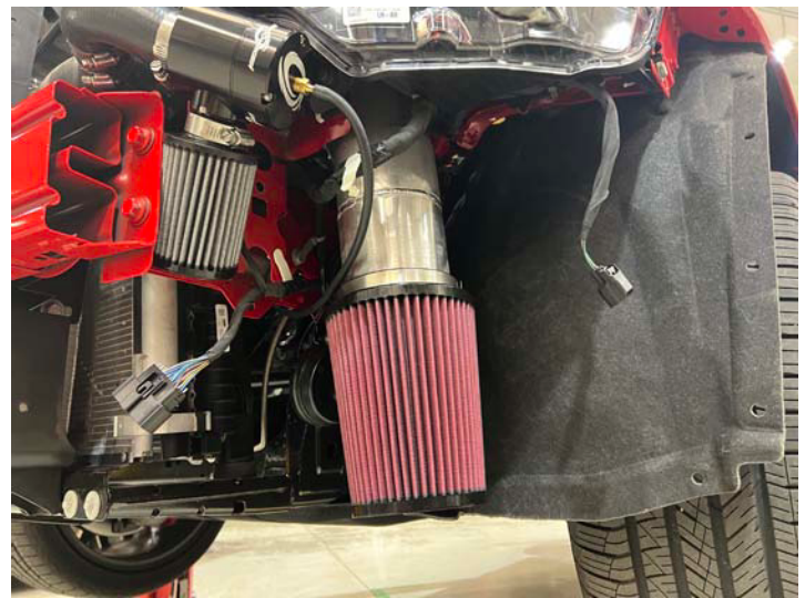
Air Inlet Installed
