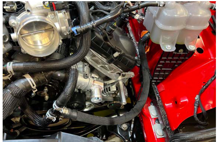
Coolant Hose Installed
