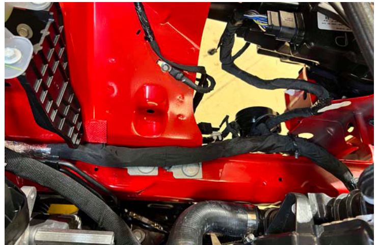
Wiring Harness Wrapped
