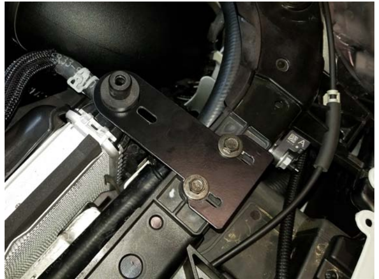
Radiator Bracket Installed
